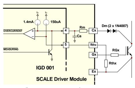
Fig. 4 Collector-sense circuit principle
