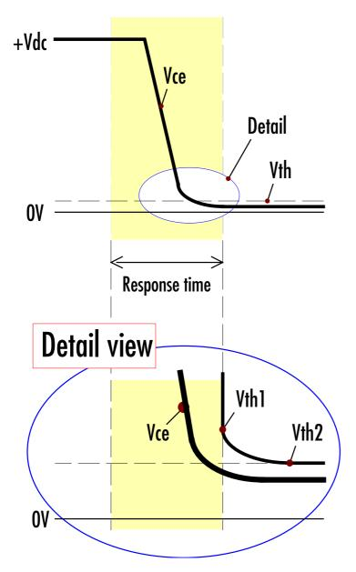
Fig. 5 Collector-sense voltage curve
